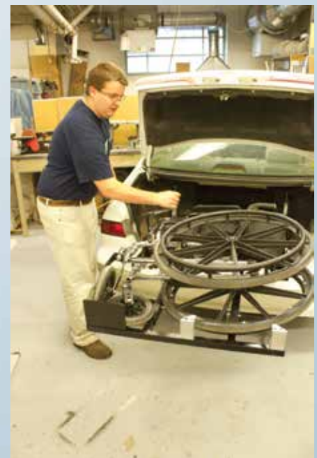
James Somers, one of the students who designed the wheelchair lift, operating the device
